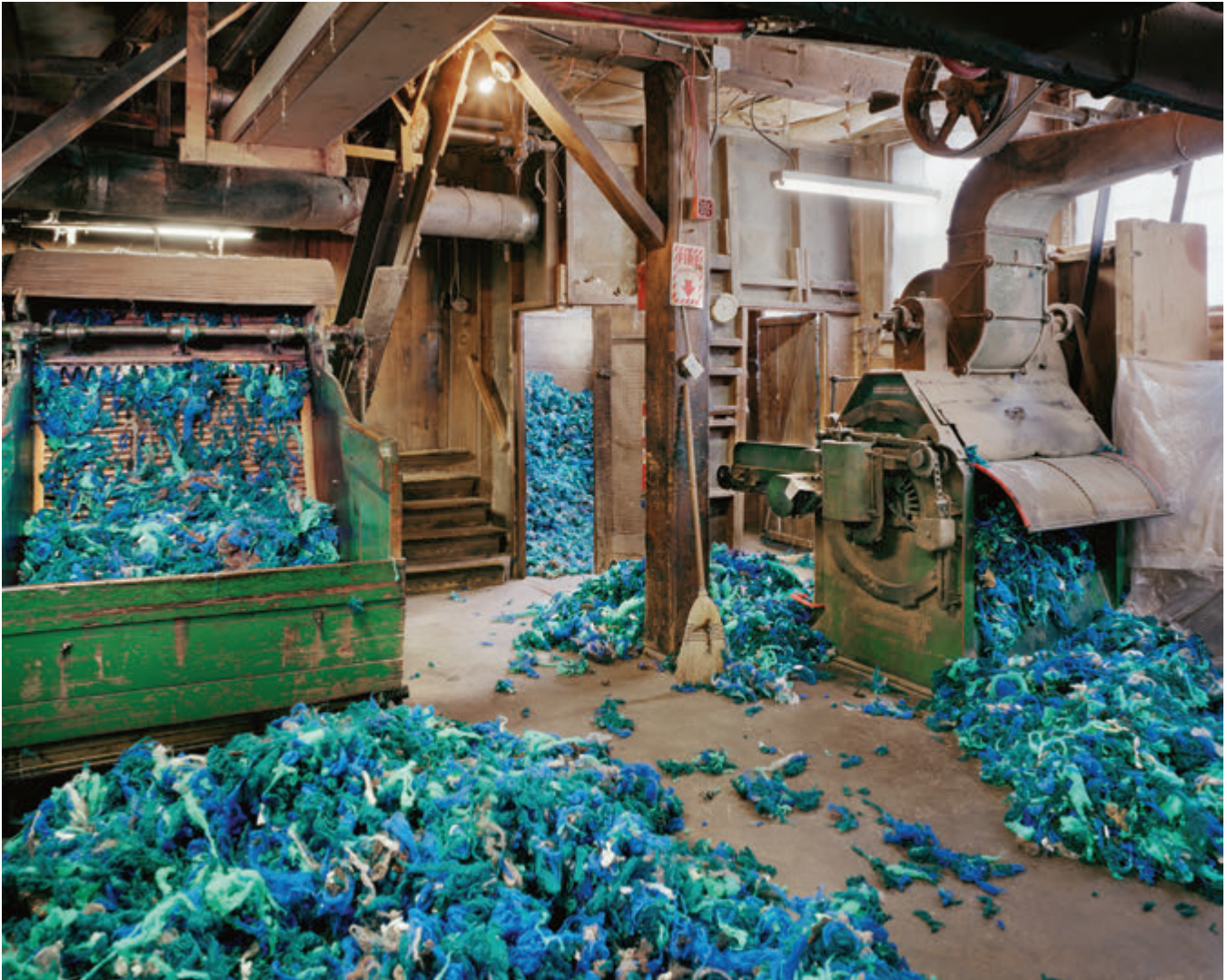
Picker and duster for separating and cleaning raw wool, Bartlettyarns, Harmony, Maine. Extruded cores for colored pencils are placed by hand in grooved wooden boards, General Pencil Company, Jersey City, New Jersey.
