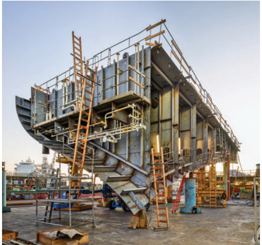
A block of container ship Matsonia under construction, General Dynamics NASSCO, San Diego. PEEPS in progress on a sugarcoated conveyor belt, Just Born Quality Confections, Bethlehem, Pennsylvania.
