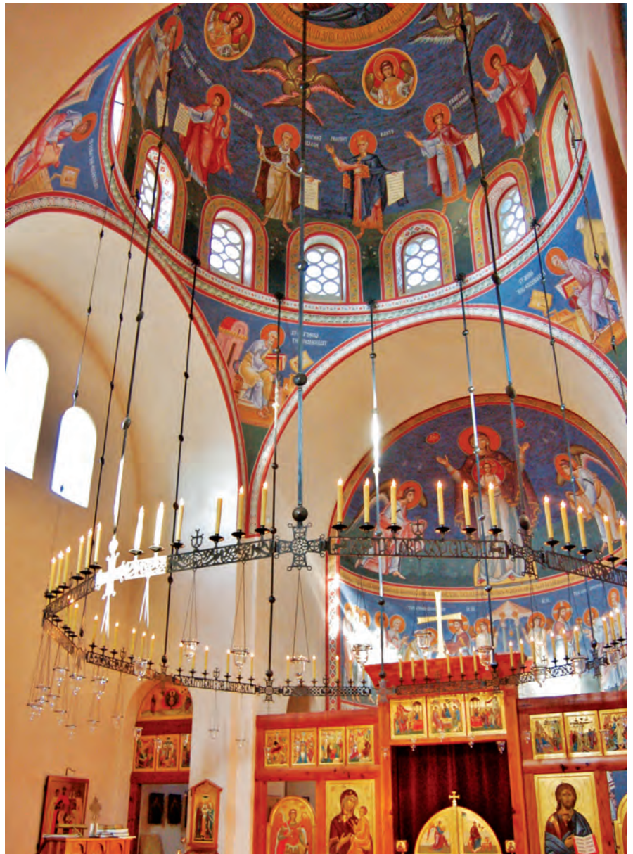
Holy Ascension Orthodox Church: Gould's first Orthodox Church features a 72-candle choros of his own design, fashioned from a steel plate using a robotic plasma cutter, and coated in an oxidized patina to approximate wrought iron.
