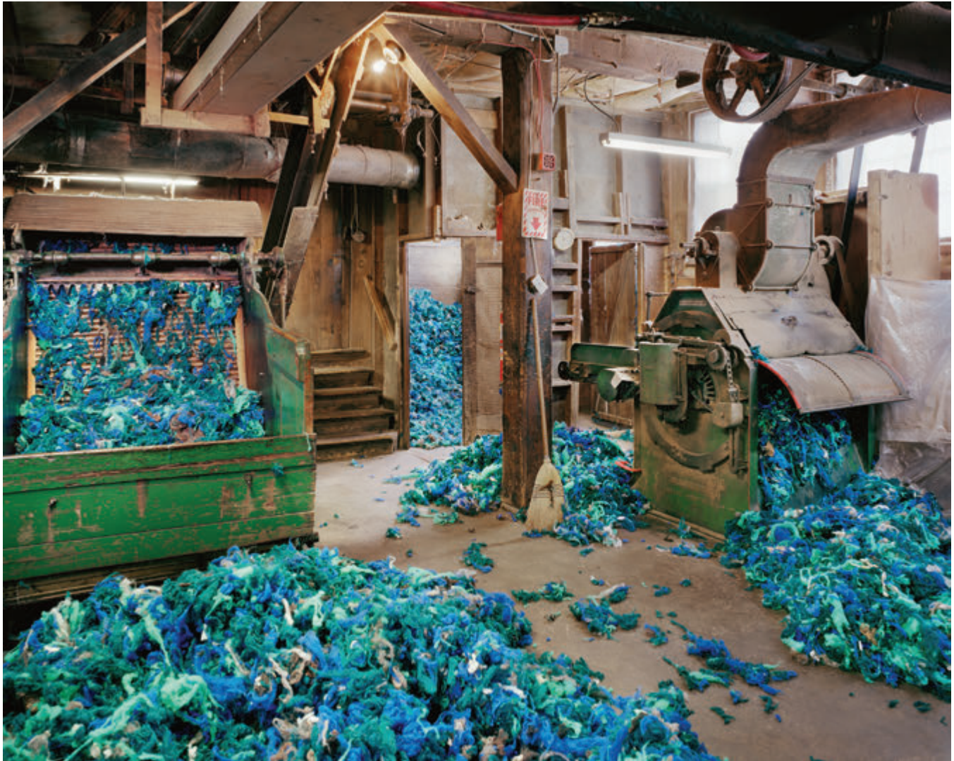
Picker and duster for separating and cleaning raw wool, Bartlettyarns, Harmony, Maine. Extruded cores for colored pencils are placed by hand in grooved wooden boards, General Pencil Company, Jersey City, New Jersey.
