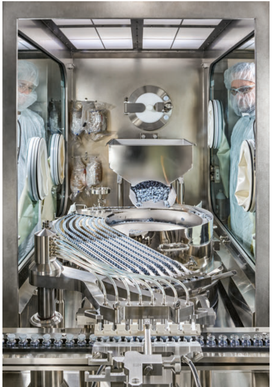
Ribbon ceramics, Corning, Inc., Corning, New York. Glass vials being filled with liquid vaccine and corked with rubber stoppers in sterile environment, Catalent, Bloomington, Indiana.
